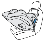
LATCH: Lower Anchor Belt DO NOT install by this method for a child weighing more than 35 lb (15.9 kg).
