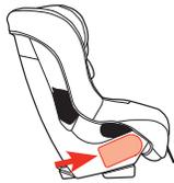
**⚠ WARNING:** Store lower anchor belt and tether strap when using the aircraft belts.
