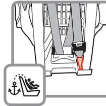
Store the tether hook when used rear facing. Attach the tether hook to storage attachment as shown.
