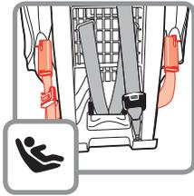
**⚠ WARNINGS:** Do not use the lower anchor belt along with the vehicle lap or lap/shoulder belt.
