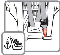
Store the tether hook when used rear facing. Attach the tether hook to storage attachment as shown.
