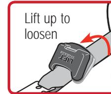
**To loosen:** Lift up on tether lock adjuster and push it towards tether hook.
