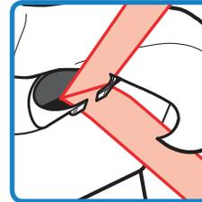
**6. You MUST Thread Only the Vehicle Lap Belt into the Belt Positioning Guides on Both Sides of the Shell As Shown**
