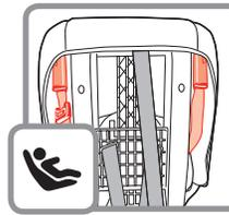
Secure the lower anchor connectors to storage attachments as shown when installing with vehicle belts.
